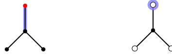
Figure 3.10: In case, the root node has only one direct child, it'll be transformed to be part of an edge block. The edge (left) and its corresponding block (right) are marked in blue. The child of the root is transformed to a vertex block with two edge blocks as children. Edge blocks are again white with black surrounding.
