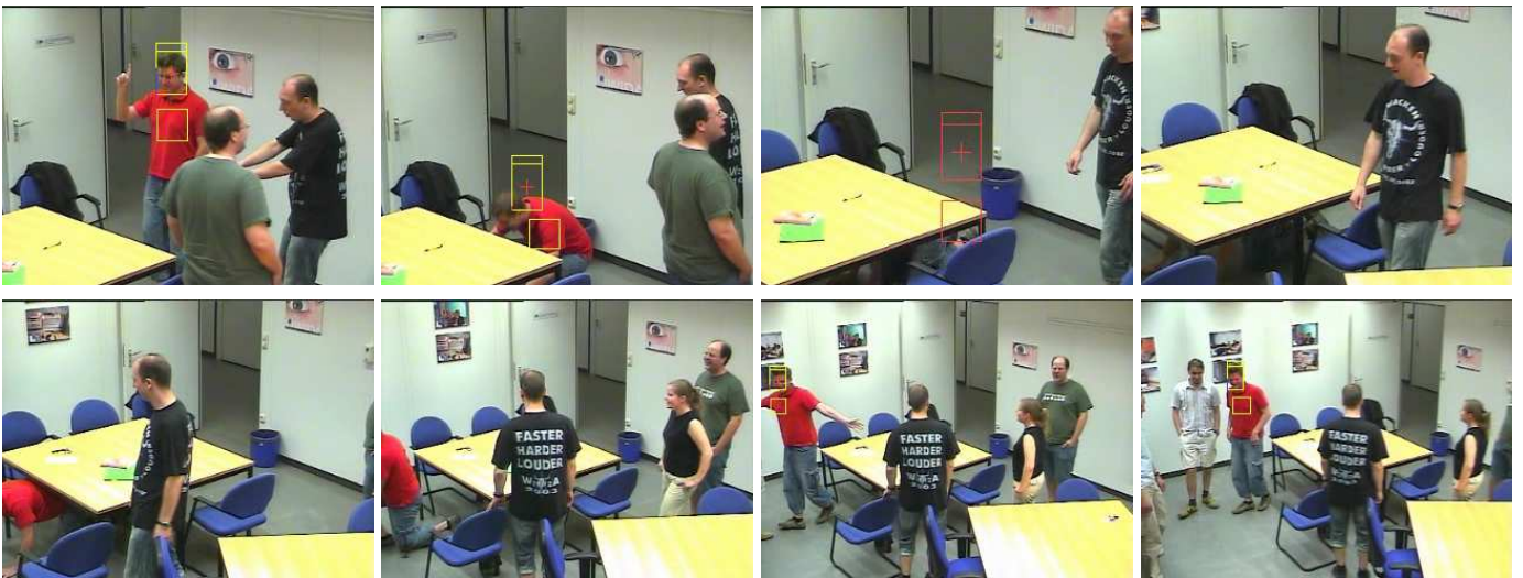
Fig. 18. Exposure to changes in camera parameters - successful relocation after zooming out. Frames t = 1350, 1375, 1400, 1425, 1450, 1475, 1502, and 1527 of sequence TS3 are shown.
