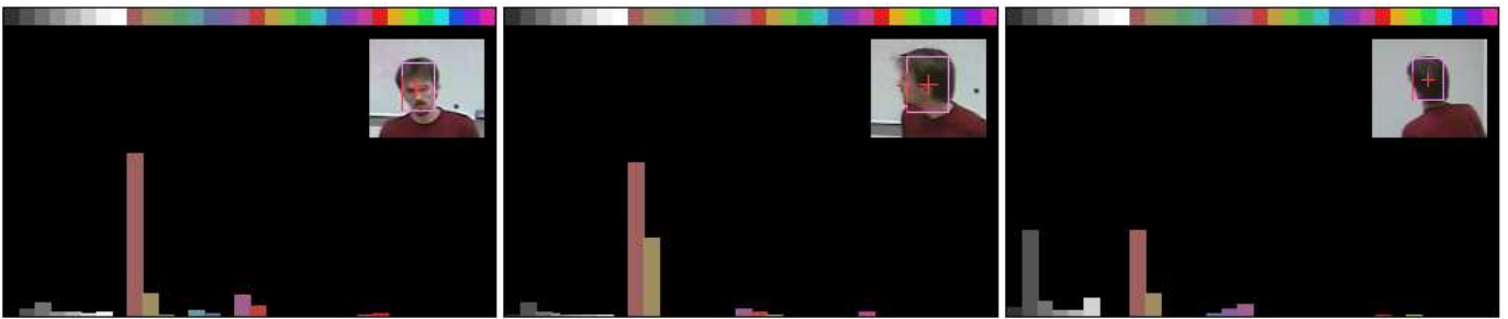
Fig. 9. Necessity for competing reference profiles. Different views of a target person imply different color distributions in the histograms.
