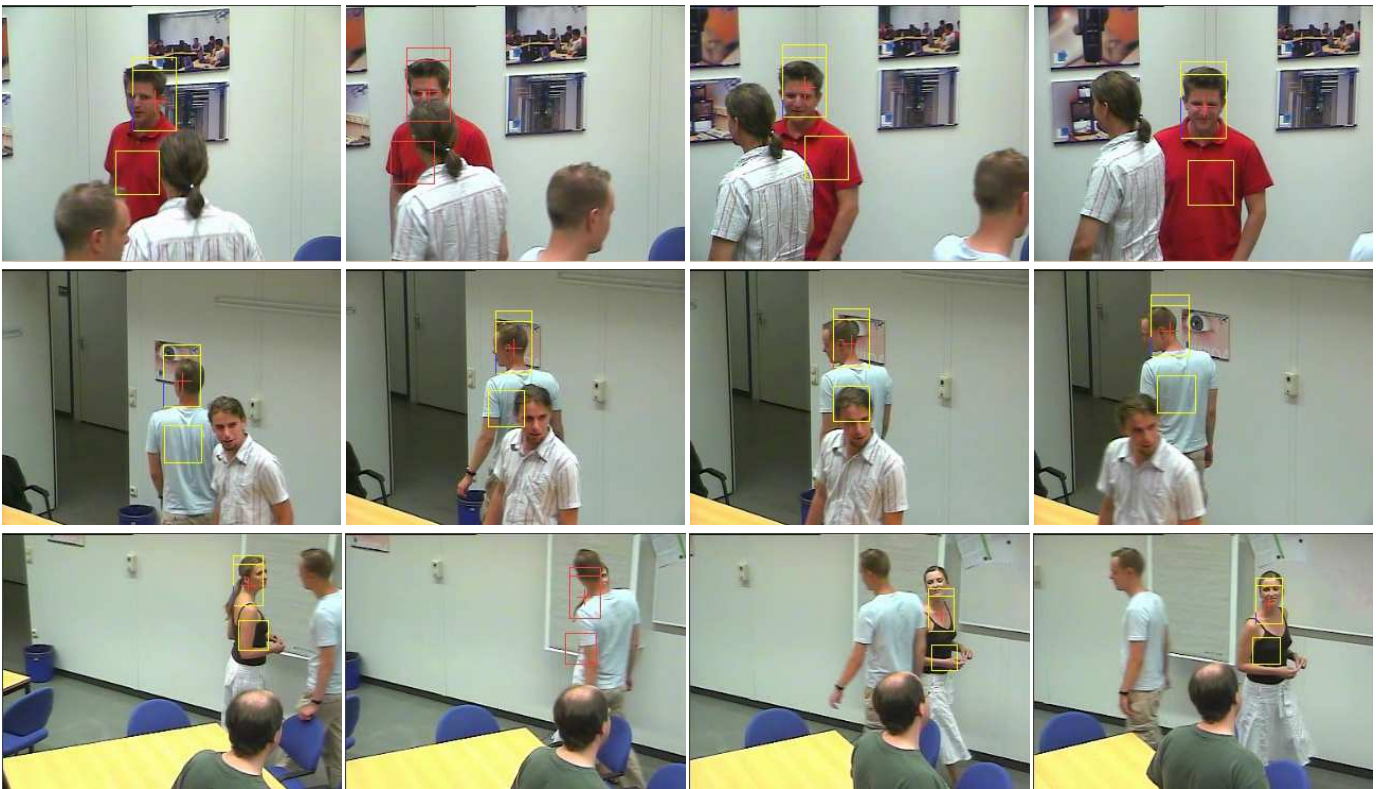
Fig. 19. Occlusions. Three sample scenes for TS3 with occlusions are shown. Upper row: frames t = 700, 717, 726, and 735 ; middle row: frames t = 2735, 2745, 2749, and 2757 ; bottom row: t = 4950, 4958, 4964, and 4975 .
