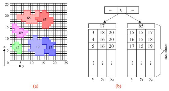
Figure 2.11: Status of a simplified map (light shaded) after applying the "deltas" at times  $t_1, ..., t_{i-1}$  to a base map BM and the changed (dark shaded) locations at time  $t_i$  (a), and the
