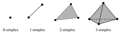
Figure 2.3: Simplex structures of different dimensions
