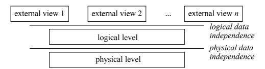
Figure 1.1: The three level architecture
