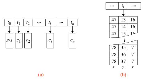
Figure 2.10: Example of an event list where  $t_i$  contains a time value (for example, day, month, and year), BM is the base map, and  $c_i$  contains all changes that occurred between the times  $t_{i-1}$  and  $t_i$  (a), structure of the changes in  $c_i$  which comprises a collection of triplets  $(x_{ik}, y_{ik}, v_{ik})$ , each of which describes the new value  $v_{ik}$  at  $t_i$  for location  $(x_{ik}, y_{ik})$  (b).
