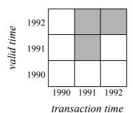
Figure 2.2: Example of a bitemporal element (BTE) [Worboys 1994 Fig. 4, used with permission.]
