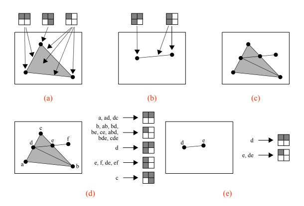
Figure 2.8: ST-complex  $C_1$  (a), ST-complex  $C_2$  (b), a common refinement of  $\pi_s(C_1)$  and  $\pi_s(C_2)$  (c), the ST-union of  $C_1$  and  $C_2$  (d), and the ST-intersection of  $C_1$  and  $C_2$  (e). [Worboys 1994, Figures 8-11, used with permission.]
