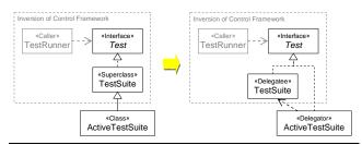
**Figure 3**. Replacing inheritance with delegation where subtyping is required (example taken from JUNIT 3.8 [16]).We will see in Section 3 that this refactoring breaks the code. Can you tell why?
