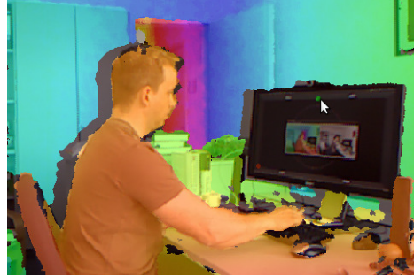
Figure 6. Merged view of colored depth-image and RGB image while selecting the second calibration sphere (green). The intended projection surface in this example is the computer display.
