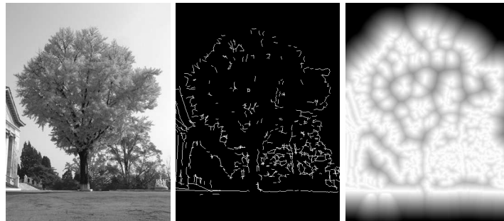
Fig. 5. Edge Image and Height Map. Left: original gray value image. Middle: binary edge image. Right: gray value height map. Note the gap in the top of the tree outline in the edge image. The height map compensates perfectly for this deficiency.
