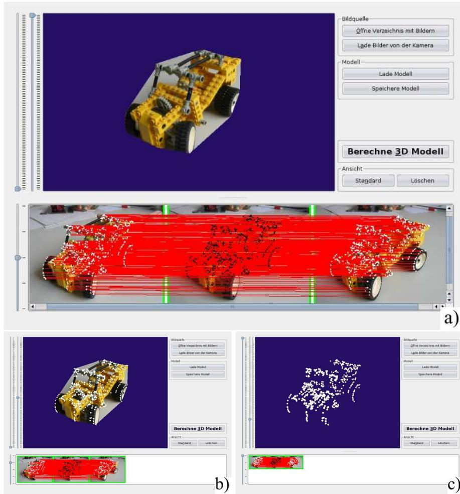
**Fig. 3.** Graphical User Interface. a) Main regions of the GUI: main window with generated 3d model, bottom window with input images and correspondences, and region with command buttons. b) Superimposition of point cloud with mapped texture, smaller display window for the loaded images. c) Main window with point cloud only, even smaller display of input images.
