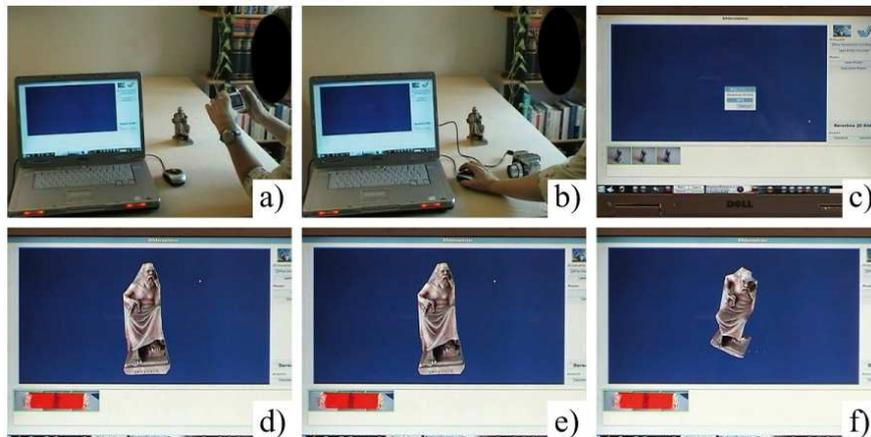
**Fig. 2.** Steps of user interaction. a) Step 1: Take snapshots. b) Steps 2, 3, and 4: Connect camera to computer, click button to initiate image loading, click button to initiate model creation. c) Progress bar is displayed. Wait a few seconds while model is generated. d) Generated 3d model is displayed. e),f) Step 5: Visualization of model from different viewpoints during rotation via mouse movement on main window.
