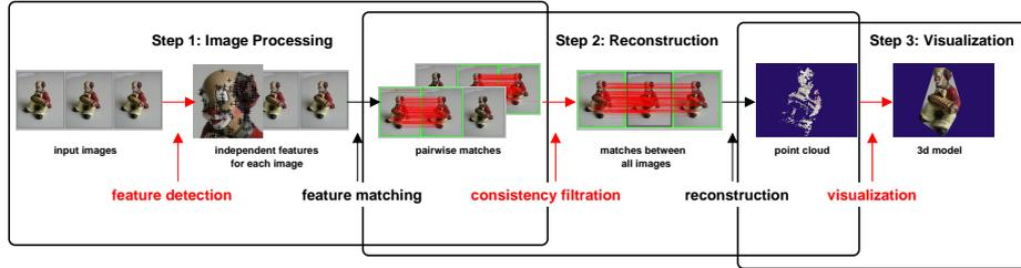
**Fig. 1.** Object acquisition pipeline. 1. Step: Image processing with feature detection and feature matching between pairs of images. 2. Step: Reconstruction with a filtration of consistent feature matches between all source images and reconstruction of the 3d positions of remaining correspondences. 3. Visualization with mapping of texture on the point cloud. Those parts of this pipeline we contribute to are highlighted in red.
