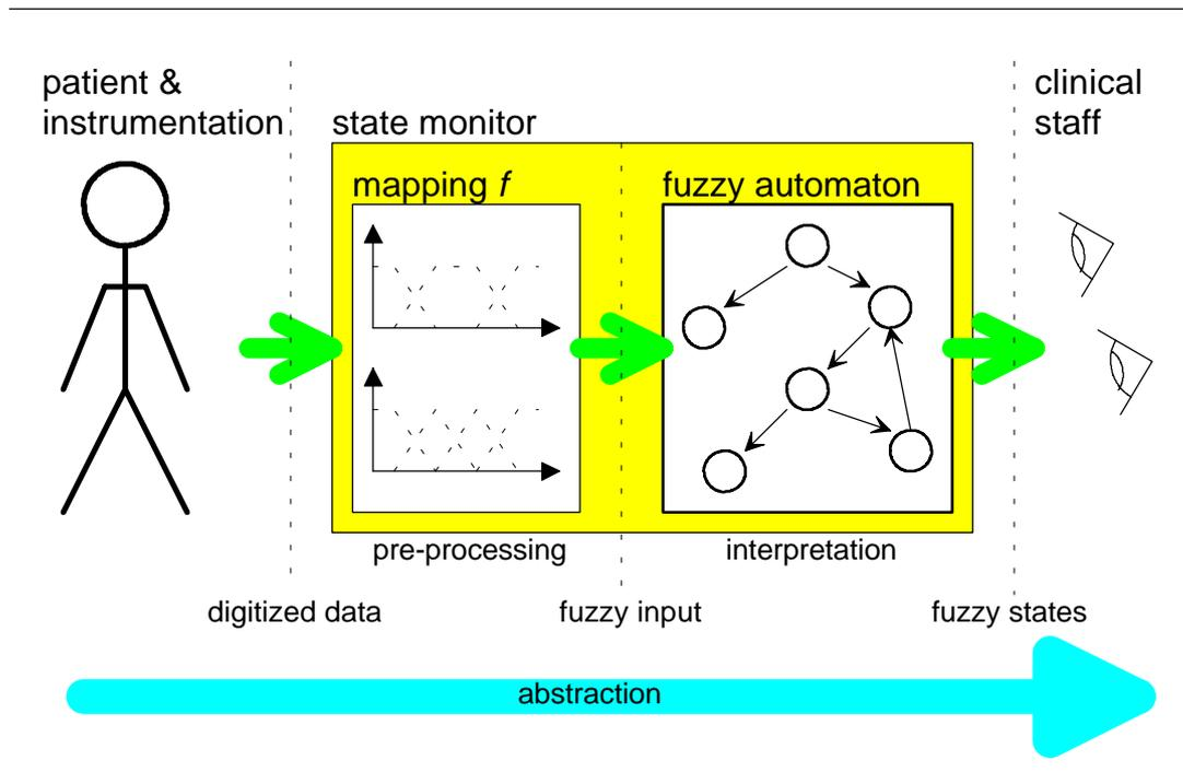
Figure 1: environment, components, and data flow of a state monitor
