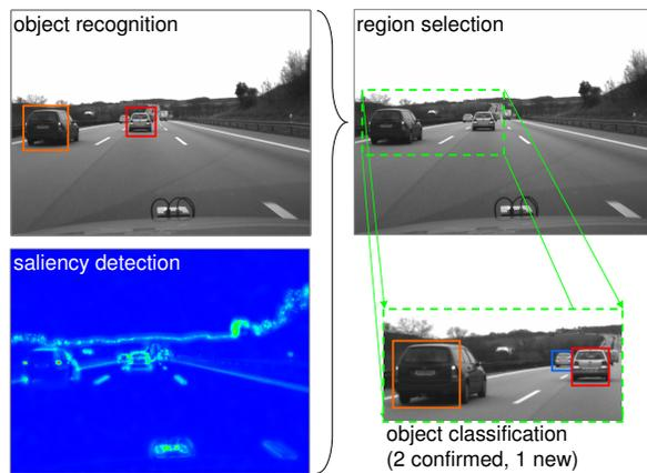
Fig. 8. Regions of interest are selected from a full video frame of a road traffic scene using our utility driven gaze control algorithm. The selective vision of a PTZ camera is emulated by extracting a  $256 \times 120$  pixel image region from a  $640 \times 480$  pixel video frame.
