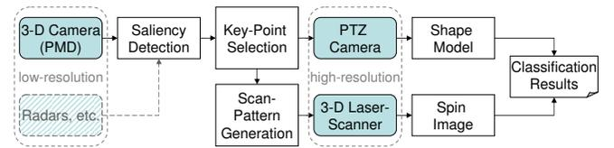
Fig. 3. Block diagram of the proposed sensor system used for object classification. Rounded boxes represent sensor resources or optional sensor resources (hatched) while rectangular boxes represent processing steps.
