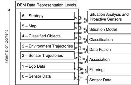
Fig. 2. Data representation levels in DEM [6]
