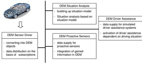
Fig. 6. Setting of the DEM evaluation
