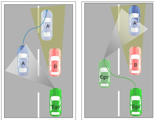
Fig. 4. Appearance and disappearance of object occlusion due to manoeuvres.
