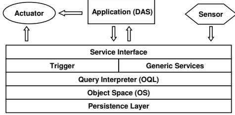
Fig. 1. Layered architecture of DEM
