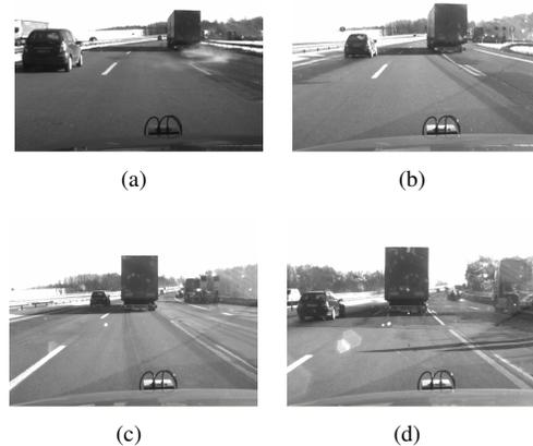
Fig. 5. Sequence of a DEM evaluation scenario which shows a critical highway scenario with a truck cutting in the ego vehicles lane and other traffic participants preventing a lane change to left.
